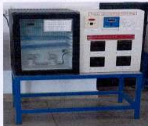
Figure 11.3 Photographic view of Refrigeration Cycle Test Rig.
