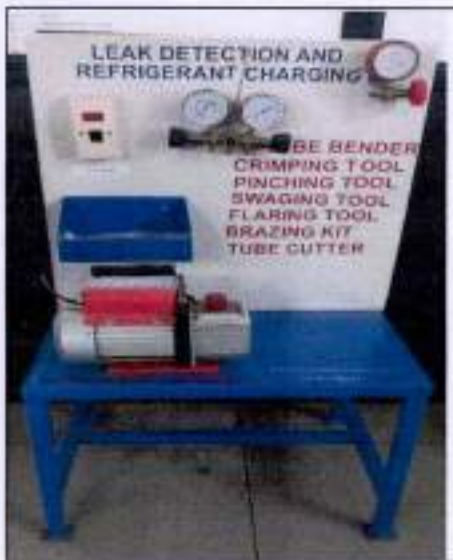
Figure 1.12 Leak Detection and Refrigerant Charging unit along with Vacuum Pump
