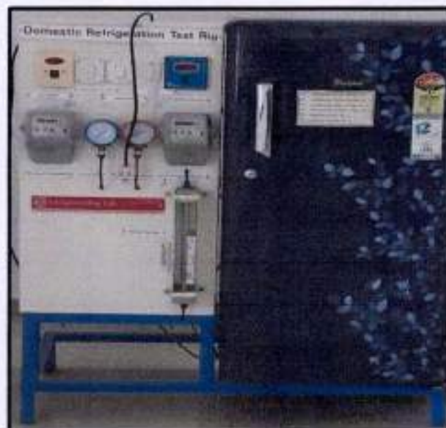
Figure 8.1 Photographic view of Refrigeration Cycle Test Rig
