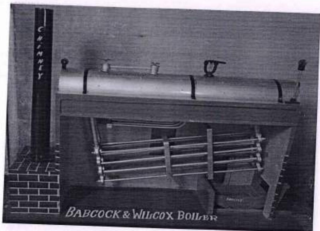
Babcock and Wilcox Boiler
